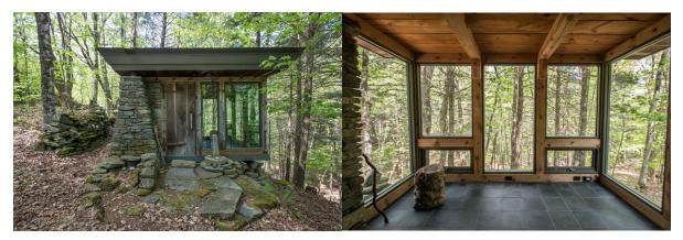
The studio, a short walk down a lovely path away from the main house, was built with timber-frame construction and fieldstone that blends into the old stone walls prevalent throughout the property. There is a slate radiant heated floor, and a threshold made of Ashfield stone "Crow's Foot."
